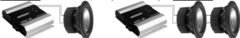
**SD700.1D/1Ω** – 4 WOOFER/4Ω OU **SD700.1D/2Ω** – 4 WOOFER/8 Ω
