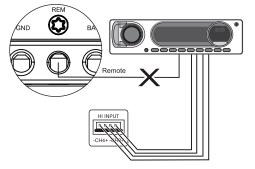
All High Signal Inputs must be connected for the 2 channels work, including the Bridge Connection
