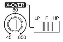
"F" All the frequencies are reproduced; "LP " Set in the variable control on Low Pass Function; "HP " Set in the variable control on High Pass Function.
