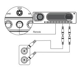
All RCA Inputs must be connected for the 2 channels work, including the Bridge Connection
