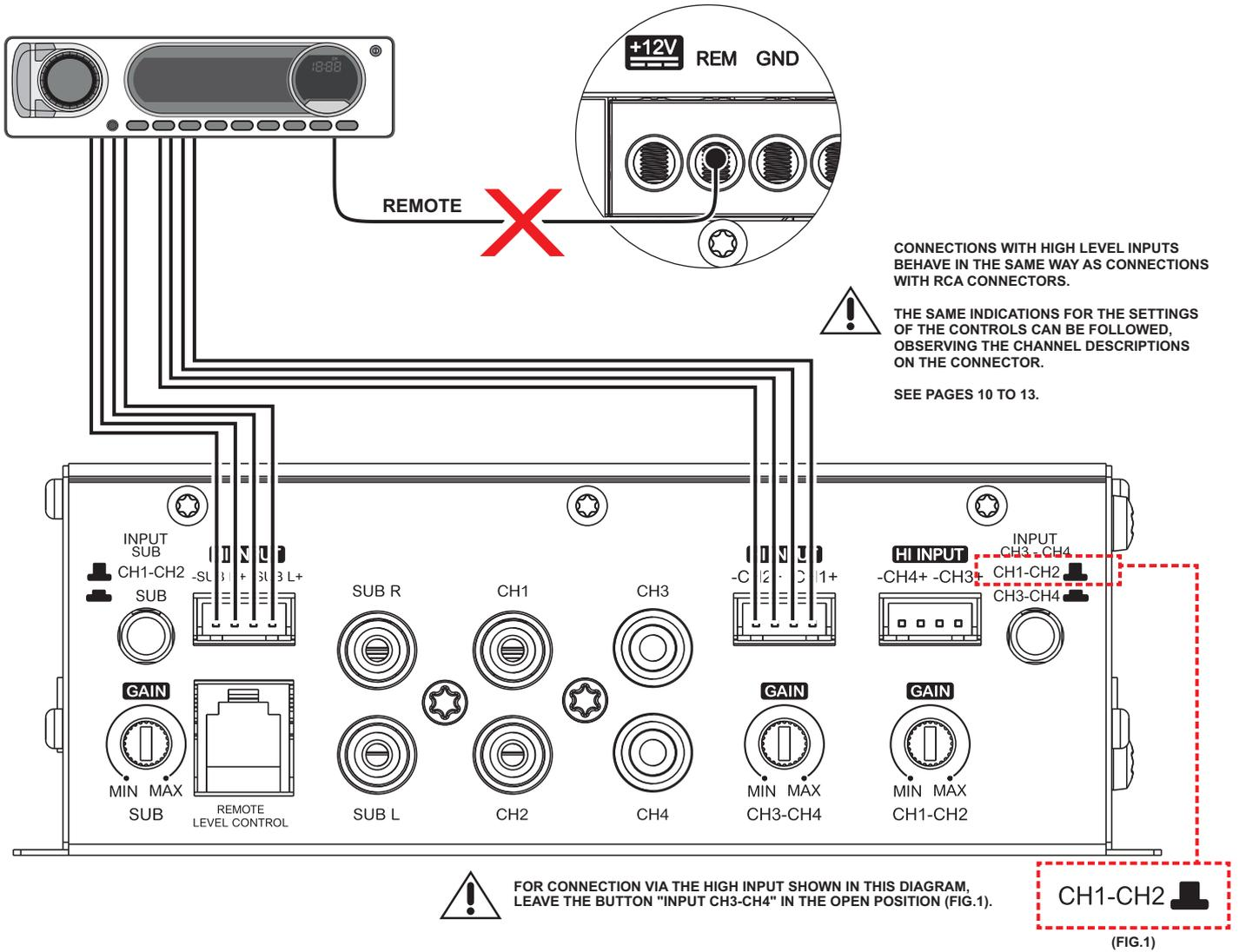
High level input must be used when the main unit does not have RCA outputs.
