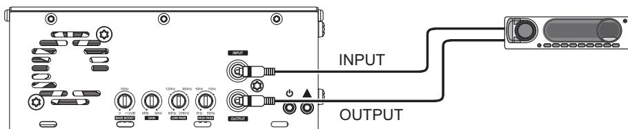
Example of one RCA cable connection only and using the RCA output to connect another amplifier.
