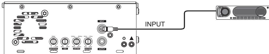
Example of two RCA cables connection (mono input).
