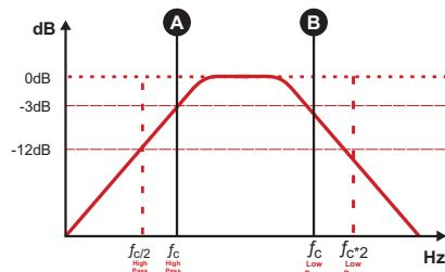
To set the "HIGH PASS" variable control between 5Hz and 80Hz ("A") where you want to perform the high pass cut filter;
