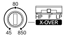
"F" All the frequencies are reproduced; "LP " Set in the variable control on Low Pass Function; "HP " Set in the variable control on High Pass Function.
