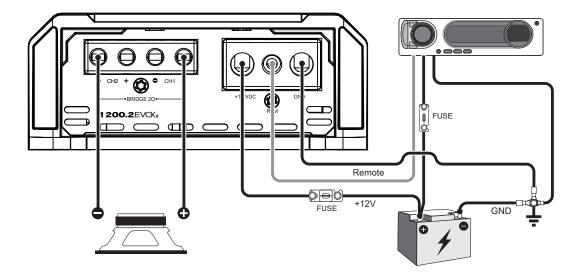
\* Check the minimum speaker impedance at specs table
