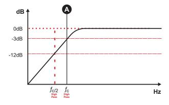
> Change the switch to "LP" position - Set in the variable control between 45Hz and 850Hz ("B") where you want to perform the low pass cut filter.
