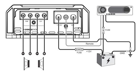
\* Check the minimum speaker impedance at specs table
