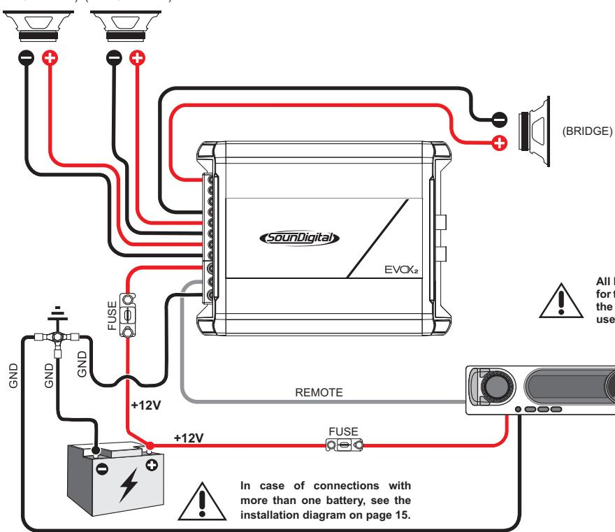
! All RCA inputs must be connected for the amplifier to work properly. If the signal source is a mono type, use a "Y" cable at the input.
