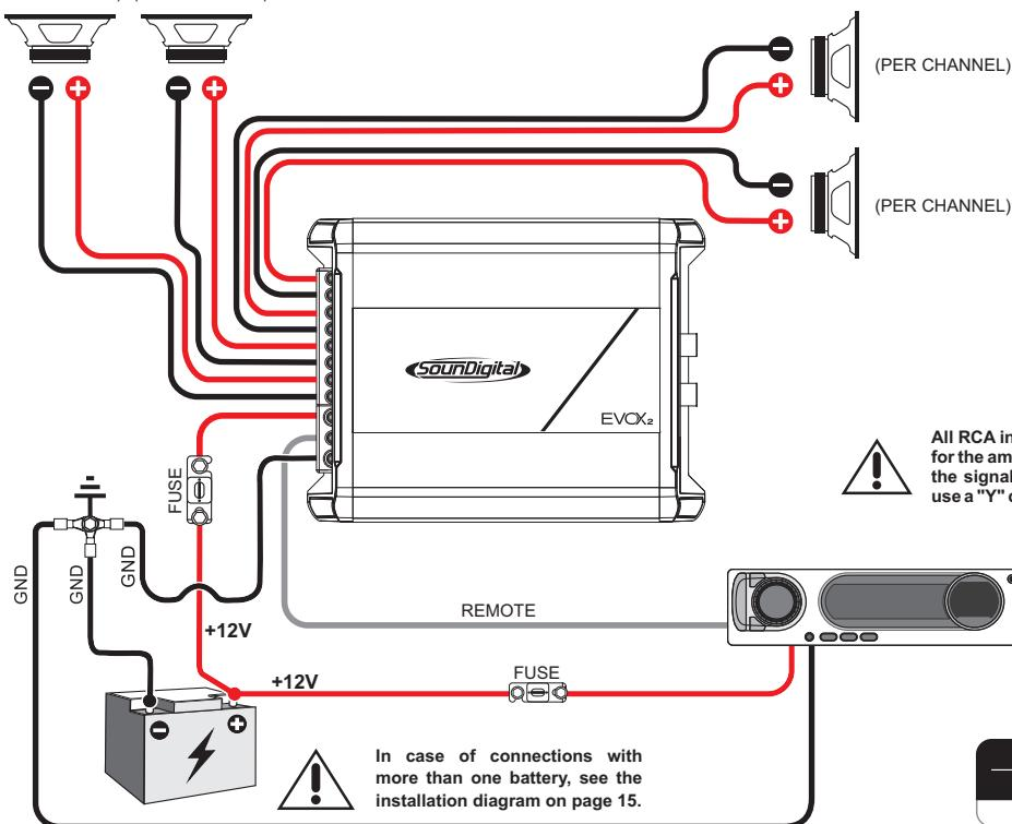
! All RCA inputs must be connected for the amplifier to work properly. If the signal source is a mono type, use a "Y" cable at the input.
