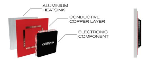
The **DTM**\* is a dynamic thermal recovery system which always maintains a high efficiency of the amplifier by accelerating the thermal exchange of electronic components with the heatsink.
