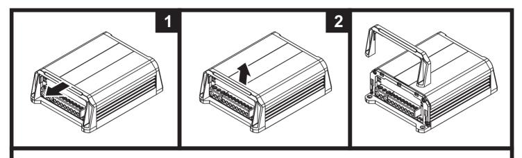
Carefully pull out the top of the plastic cover to release the upside latches, as shown in picture 1.
