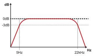
> Change the switch to "HP" position - Set in the variable control between 45Hz and 850Hz ("A") where you want to perform the high pass cut filter;
