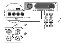
All RCA inputs must be connected for the amplifier to work properly. If the signal source is mono type, use "Y" cable at the input.
