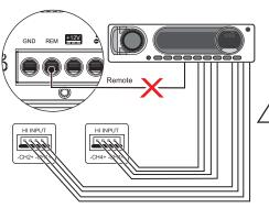
All High level signal inputs must be connected for the amplifier to work properly.
