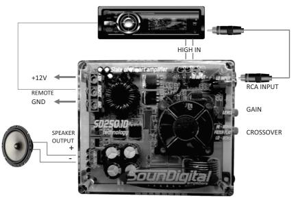
Warning: Never use the high in input and RCA input together. If the main unit have RCA output, use only this ouput, if doesn't have, use the high output.
