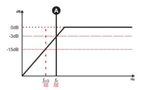
Use in Band Pass Mode - adjust the "HIGH" control - "A" frequency between 5 Hz and 30 Hz and the "LOW" control - "B" frequency between 50 Hz and 500 Hz.
