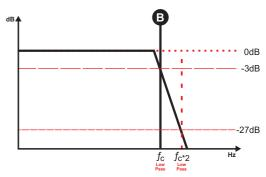
Use in 12dB/Oct Low Pass Mode - adjust the "HIGH" control to 5 Hz, and the "LOW" control, the "B" frequency between 50 Hz and 500 Hz.
