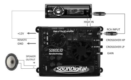
Warning: Never use the high in input and RCA input together. If the main unit have RCA output, use only this ouput, if doesn't have, use the high output.
