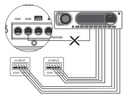
All High signal Inputs must be connected for the 4 channels to work.
