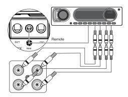
All RCA Inputs must be connected for the 4 channels to work.
