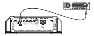
Example of two RCA cables connection (mono input).
