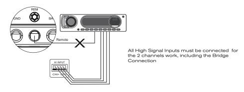
High input must be used when the main unit does not have RCA outputs.
