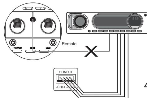
All High Level Inputs must be connected for the all channels to work properly.
