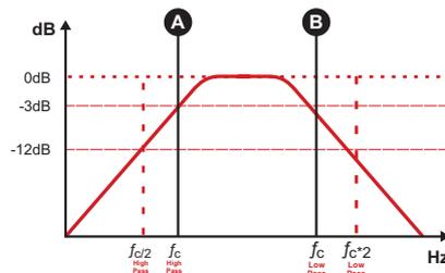
To set the "SUBSONIC" variable control between 5Hz and 80Hz ("A") where you want to perform the subsonic cut filter;
