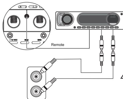
All RCA Inputs must be connected for the all channels to work properly. If the signal source is mono type, use "Y" cable at the input.
