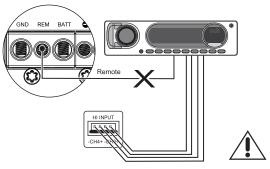
All High Level Inputs must be connected for the all channels to work properly.
