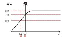
Set in the "LOW" variable control between 50Hz and 20kHz ("B") where you want to perform the low pass cut filter;
