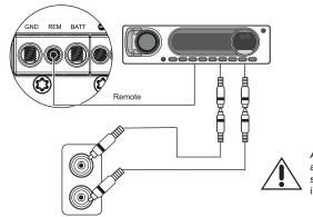
All RCA Inputs must be connected for the all channels to work properly. If the signal source is mono type, use "Y" cable at the input.
